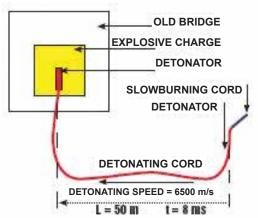
Picture 6. Scheme of the possible destruction of the bridge
